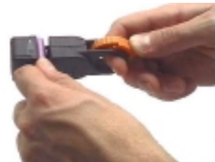
3. Insert the measured end of the cable into the tool as far as allowed by the index finger of the left hand.
