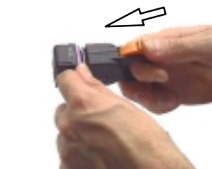
4. Clamp the end of the cable in the stripping tool.
