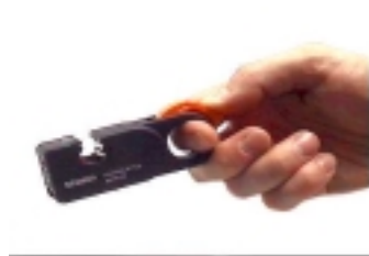
1. How to hold the stripping tool in the right hand
