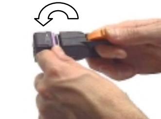
5. Turn the tool four times in the direction of the arrow for PVC insulation (eight times for PUR or PE insulation).
