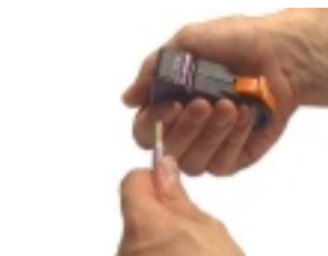
7. Remnants remain in the tool. After opening the tool, the remnants of the cable can be removed.
