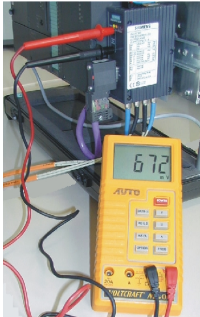
Figure A-6 Testing the Signal Quality on an OLM V3 with a Voltmeter
