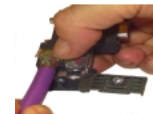
9. Fit the FastConnect cable into the connector.
