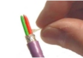
8. Remove the protective layer from the cores.
