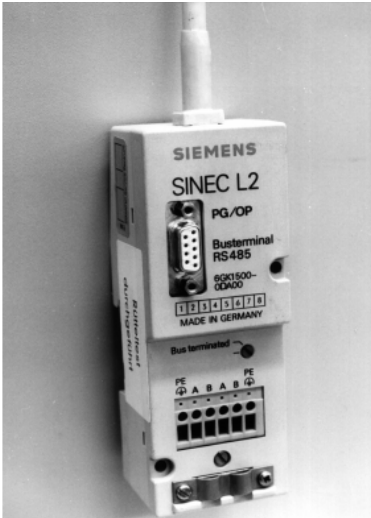
Figure 4-28 RS-485 Bus Terminal with Additional PG Interface
